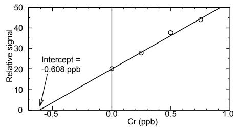
Multiplying the *x*-intercept by  $2.00 \times 10^5$  tells us that the soil contains 122 ppm of Cr(VI).
