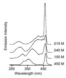
Concentration dependence of fluorescence intensity of biacetyl in CCl<sub>4</sub> with  $\lambda_{ex} = 422 \text{ nm}$  and  $\lambda_{em} = 464 \text{ nm}$ . [From G. Henderson, J. Chem. Ed. **1977**, 54, 57.]
