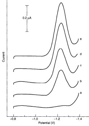
Anodic stripping voltammograms of Cr(VI) from contaminated soil from K. B. Olsen, J. Wang, R. Setladji, and J. Lu, *Environ. Sci. Tech.* **1994**, 28, 2074.
