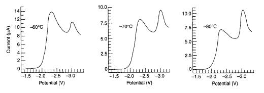
Voltammograms of 2.0 mM *trans*-1,2dibromocyclohexane at a frozen mercury-drop electrode in butyronitrile with 0.10 M (*n*-C4H9)4NCIO4 electrolyte. Scan rate = 1.00 V/s. (D.H. Evans, K.M. O'Connell, R.A. Petersen, and M.J. Kelly, *J. Chem. Ed.* **1983**, 60, 290.)
