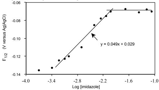
Dependence of half-wave potential (measured by cyclic voltammetry) on ligand concentration for reduction of  $Fe^{3+}$  complex to  $Fe^{2+}$  complex. [Data from D. K. Geiger. E. J. Pavlak and L. T. Kass, *J. Chem. Ed.* **1991**, *68*, 337. This article describes a student experiment for measuring binding constants.]
