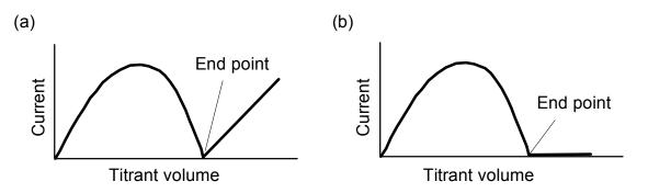
Now consider what happens when  $S_2O_3^{2-}$  is added to  $I_2$ . At first, no I<sup>-</sup> is present and only residual current is observed. As the reaction proceeds, I<sup>-</sup> is created and current is conducted between the two polarizable electrodes by means of the following reactions:
