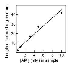
Calibration graph for Al<sup>3+</sup> using tube containing Alizarin Red S.
