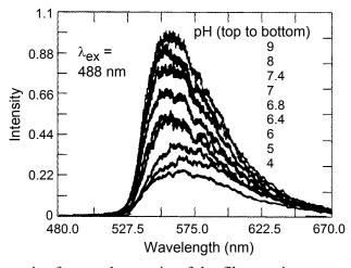
Fluorescence intensity from polymer tip of the fiber optic sensor shown at the beginning of Chapter 10. [From W. Tan, S.-Y. Shi, S. Smith, D. Birnbaum and R. Kopelman, *Science* **1992**, *258*, 778.]
