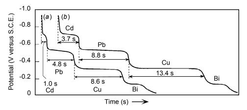
Potentiometric stripping curves from a sample containing  $Cd^{2+}$ ,  $Pb^{2+}$ ,  $Cu^{2+}$  and  $Bi^{3+}$  (*a*) before and (*b*) after addition of 0.5 µg/L of  $Cd^{2+}$ ,  $Pb^{2+}$ , and  $Cu^{2+}$ . There was no dilution caused by the standard addition. The sample contained 0.5 M NaCl, 0.05 M HCl, and 1 mg of Hg<sup>2+</sup>/L. [From L. D. Jagner, *Anal.. Chem.* **1978**, *50*, 1924.]
